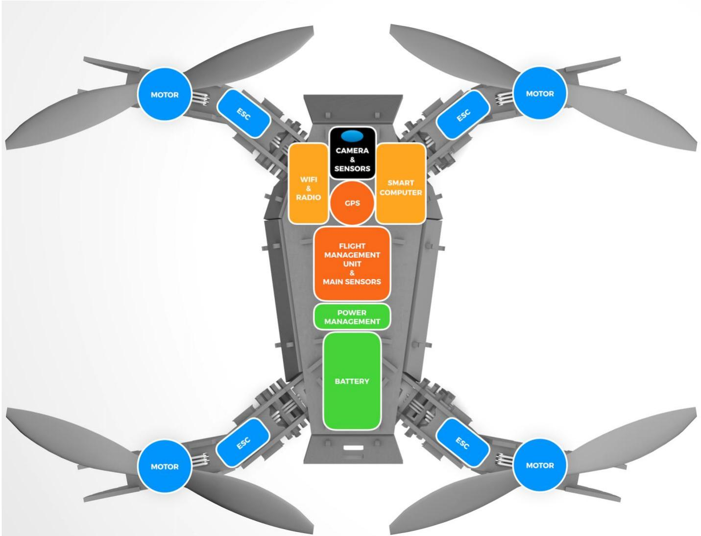
A typical drone air vehicle consists of:
