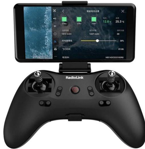
Smartphones and tablets are the most commonly used displays for seeing the flight information, camera feeds, and providing menus of services. They provide all of these and additional communications links like bluetooth and WiFi. Other times, the display is built into the hand-held flight controller.
