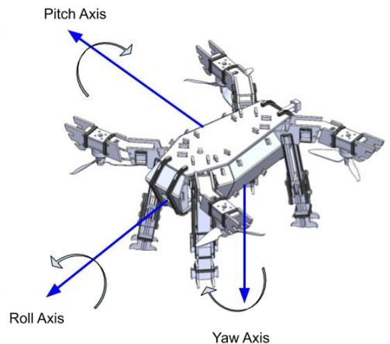
Positive roll is rolling to the right, lifting the left wings and lowering the right wings (clockwise) around this axis. Positive pitch is rotating (or pitching) up which raises the nose and lowers the tail (clockwise) around this axis. Positive Yaw is where the drone's nose turns to the right, or clockwise around this axis.
