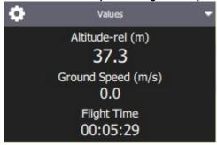
c. You can configure what information is displayed by pressing the small gear icon on the top left of the panel. Each value can be displayed in normal or "large" size (large size shows just one value per row in the page, while normal shows 2).
